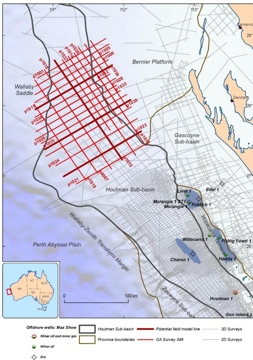
**Figure 1:** Location of the GA349 regional seismic survey (red lines) along the West Australia Margin, overlain on digital elevation model. Wells and hydrocarbon shows are shown on the map. Location of structural and basin elements are labelled in italic. Thick red lines represent potential field model lines undertaken during this study to test structural seismic interpretation and developed a crustal model. The line 1031 is shown in Figure 3.
