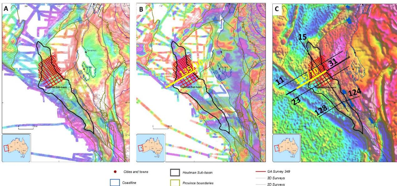
**Figure 2:** A and B - Merged gravity and magnetic anomaly dataset with ship track data distribution (Transparent red lines) (from Hackney, 2012). C - Satellite FA gravity data (Sandwell and Smith, 2009) including location of the GA349 regional seismic survey (red lines) and gravity modelling profiles in the Houtman Sub-Basin. Black lines show the location of gravity model profiles and the yellow line indicates the magnetic model profile location.
